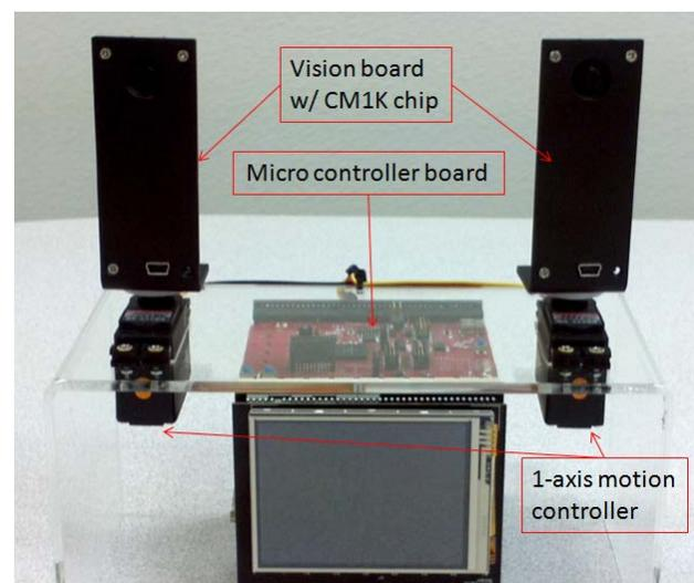
The stereo vision algorithm can be decomposed into three phases as described below and the CogniMem (CM1K) chip offers essential benefits in each phase.
