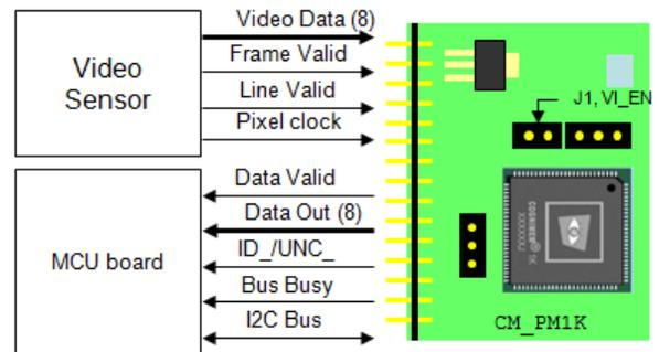
The next diagrams illustrate different options to recognize an object in your video images. First, the real-time recognition logic is enabled by settings bit 0 of the RSR register to 1. The recognition starts immediately at the next Frame Valid pulse and applies to the default region of interest defined in the CM1K. This region occupies 1/3 of the video frame and is centered in the video frame.
