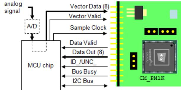
The next diagrams illustrate different options to obtain the classification of the Vector Data. First, the real-time recognition logic is enabled by settings bit 0 of the RSR register to 1. The recognition starts immediately at the next Vector Valid pulse.
