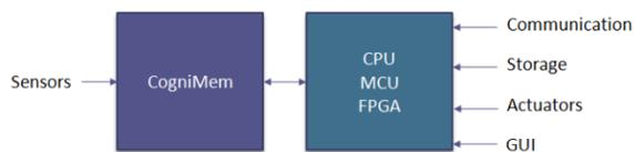
Beyond the arena of the low-cost, low-power embedded systems, multiple CogniMem chips can be daisy-chained to build massively parallel data mining systems with unlimited capacity and a recognition time independent of the size of the knowledge base.
