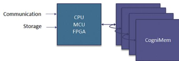
Building banks of CogniMem chips is effortless. On the hardware side, it simply requires daisy-chaining the chips and connecting them together through their parallel bus. On the firmware side there is no impact whether your hardware uses a single chip or a bank of many
