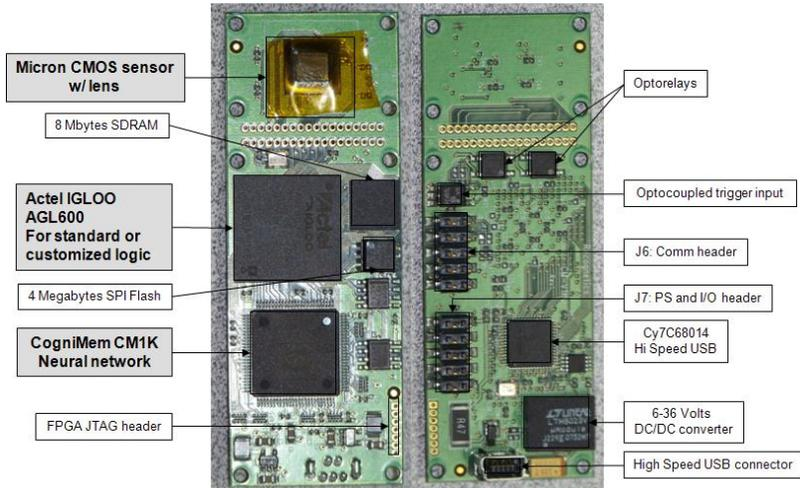
Access to all the components of the board is made via a simple Register Transfer Level (RTL) protocol. The CogniMem chip can be used independently from the recognition engine, to learn and recognize vector data transmitted from a host. FPGA programmers can implement their own feature extraction, results conditioning, and transmission to run on the board as an embedded platform.
