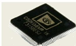
CM1K features 1024 cognitive memories, or neurons, working in parallel and capable of learning and recognizing patterns of up to 256-bytes in a few microseconds. The parallel architecture of CM1K allows to daisy-chain many chips together to increase the size of the memory bank, or neural network, by increment of 1024. Its low pin-count and low power consumption make it an ideal companion
